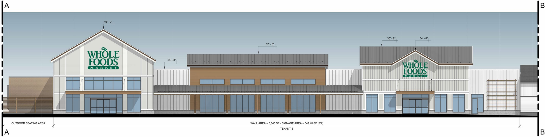
② ELEVATION BUILDING B 3/32" = 1'-0"
